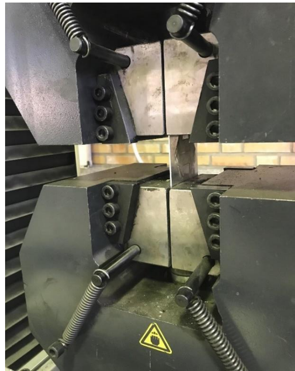
Fig.2. Specimen Positioning in the Load-Cell
