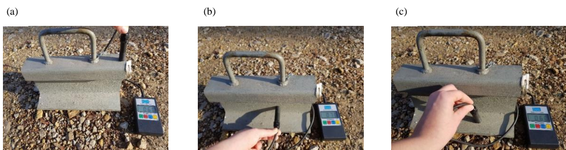
Fig. 5. Measurement of the paint film thickness on a rail type S49 (49E1) (own photograph): (a) on the head/crown of the rail; (b) on the neck; (c) on the foot
